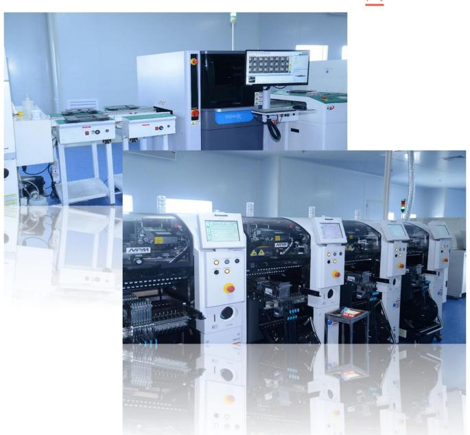
Small-pitch products demand extremely high specifications on the efficiency and accuracy of the placement machines. We facilitate a new type of high-speed placement machines throughout the whole line, which for fill this requirements.
